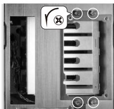
Loos four thumb screws to remove the PSU mounting bracket.
