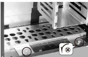
Loose thumb screws to remove the 2.5" / 3.5" HDD tray.
